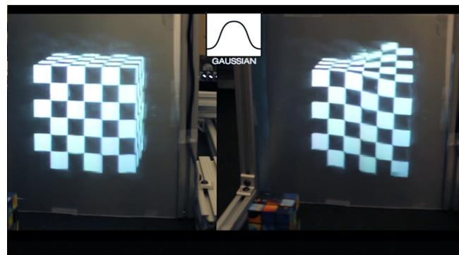
**Video 5** Assuming a constant viewer height per projector frame causes image tearing and distortion (right). Per-vertex height interpolation allows for a consistent perspective (left) [URI: <http://dx.doi.org/10.1117/1.JEI.23.1.011005.5>].
