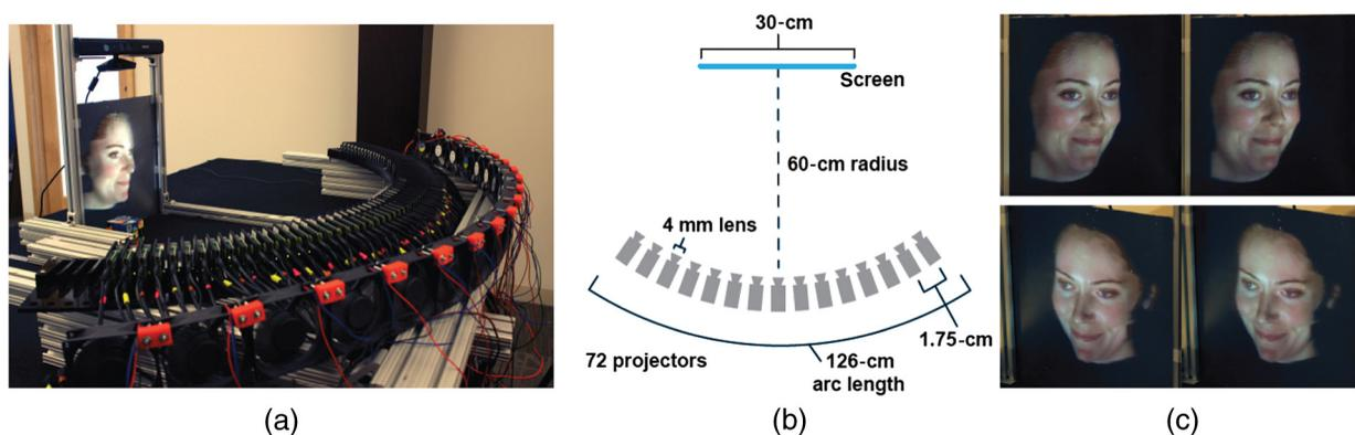
**Fig. 1** (a) A three-dimensional (3-D) face is shown on our autostereoscopic 3-D projector array. The display combines both autostereoscopic horizontal parallax with vertical tracking to generate different horizontal and vertical views simultaneously over a full 110-deg field of view. (b) Diagram showing the dimensions of the display. (c) 3-D stereophotographs of a human face. The stereopairs are left-right reversed for cross-fused stereoviewing.
