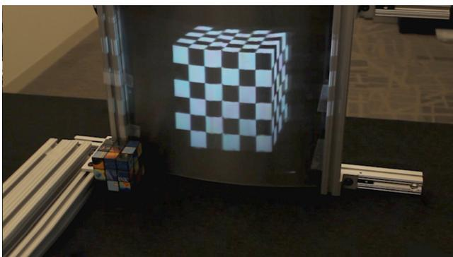
**Video 4** Vertical parallax is shown for a tracked viewer and a curved front-projection screen. The reflected projector positions are iteratively refined to correct for the mirror shape (MOV, 2.66 MB) [URI: <http://dx.doi.org/10.1117/1.JEI.23.1.011005.4>].
