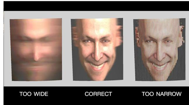
**Video 7** Simulation of screens with different levels of horizontal diffusion. The ideal horizontal diffusion should match the angular spacing between projectors [URI: <http://dx.doi.org/10.1117/1.JEI.23.1.011005.7>].
