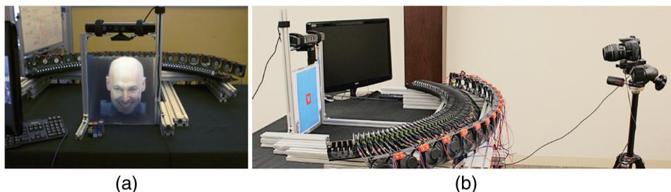
**Fig. 3** (a) Photograph of our rear-mounted projector array setup. (b) Photograph of the calibration setup for front-mounted projector array. To compute relative projector alignment, we sequentially correspond a virtual AR marker generated by each projector with a printed AR marker.
