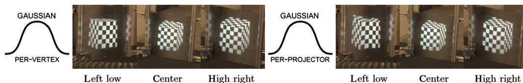
**Fig. 9** Comparison of different viewer interpolation functions for a convex mirror. The left set uses per-vertex viewer height and distance with a Gaussian falloff. The right set uses constant height and distance per projector with a Gaussian falloff. Photographs taken with per-vertex interpolation show less distortion with consistent vertical perspective. In contrast, straight lines appear curved in photographs using constant per-projector interpolation.
