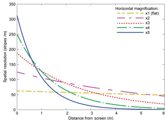
**Fig. 6** Graph showing tradeoff between spatial magnification using convex mirrored screens and depth of field. Greater mirror curvature increases density of projector stripes and spatial resolution at the screen; however, spatial resolution falls off rapidly away from the screen.
